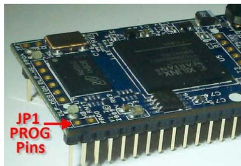
The user must hold the short across the PROG pins in place while using the BitLoadApp to write a valid configuration file into the SPI flash. When the write is complete, just remove the short, and the FPGA configuration will succeed. At this point, the BitLoadApp will work properly.
