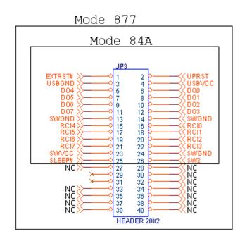
Connection to target electronics is made a 40-pin connector (JP3), however only 26 pins of the connector are used by the DLP-IO16.
