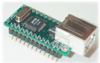
To send data from the peripheral to the host computer simply write the byte wide data into the module when TXE#
