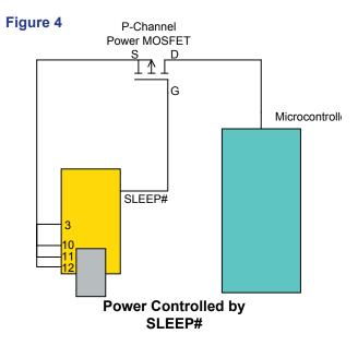
recommend that a dedicated power switch i.c with inbuilt "soft-start" is used instead of a MOSFET. A suitable power switch i.c. for such an application would be a Micrel (www.micrel.com) MIC2025-2BM or equivalent.
