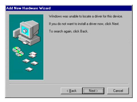
The most common reason for this is that the VID and PID values in the INF files do not match those of the hardware. If you have changed the VID and PID of the product using FTDI's E2PROG utility then you need to add entries in the INF files to match the new VID and PID.
