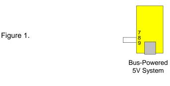
The figure above illustrates a typical USB bus-powered configuration. A USB bus-powered device gets its power from the USB bus.
