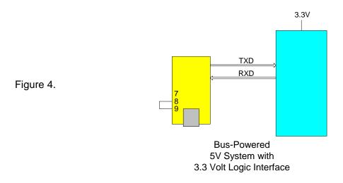
Figure 4 shows how to configure the DLP-USB1232H to interface with a 3.3V logic device via the ASYNC serial mode. In this example, the target electronics provide the 3.3 volts to power the microcontroller.
