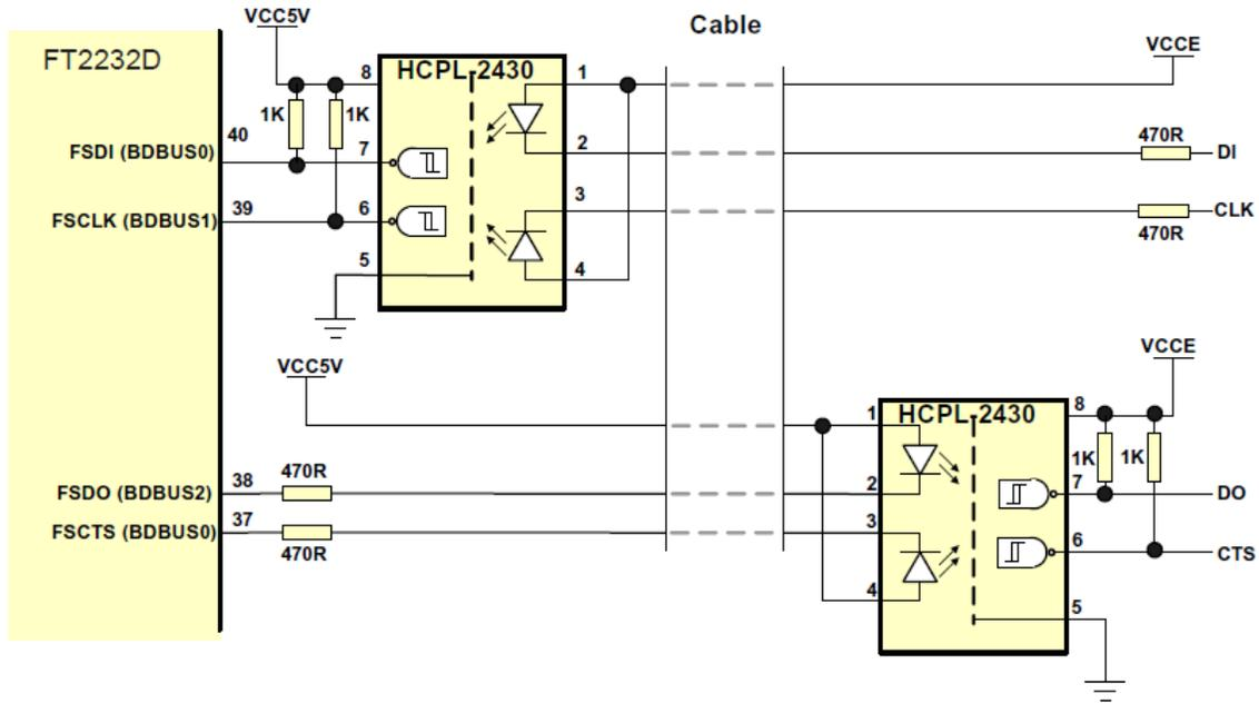
Figure 36 - Fast Opto-Isolated Serial Interface Example
