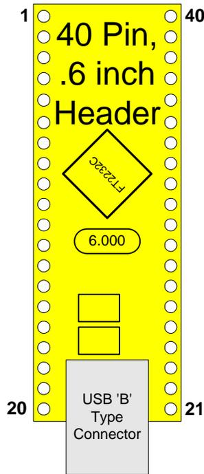
Figure 2. Pin-Out (40 Pin DIP Header )
